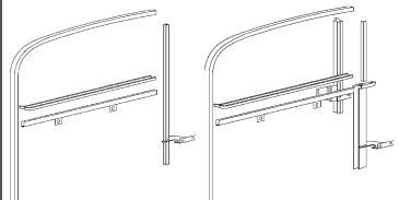
Kits include all felt channels, window bottom felt, and vent window division felt, installation clips, and screws for 2 windows. Kits do not include felt strip for front vent divider stainless frame strip.
